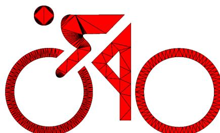
**Figure 10 Zones in a triangulation**
